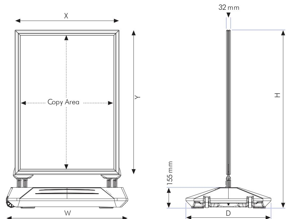
Pavement board with 40 mm alu snap-frame cut in mitred with rounded corners. Antireflex APET front panels. Mounted with black rubber to protect the poster from water. Springs are treated to prevent corrosion. The foot is made of heavy duty plastic material and can be filled with water or sand to give the sign a really good stability even in rough weather conditions. Please add anti-freeze if below 0° C degrees. The two wheels makes the board easy to move around. Easy and fast to assemble.
